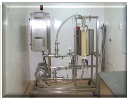
Ultrafiltration System for tangential ultrafiltration
